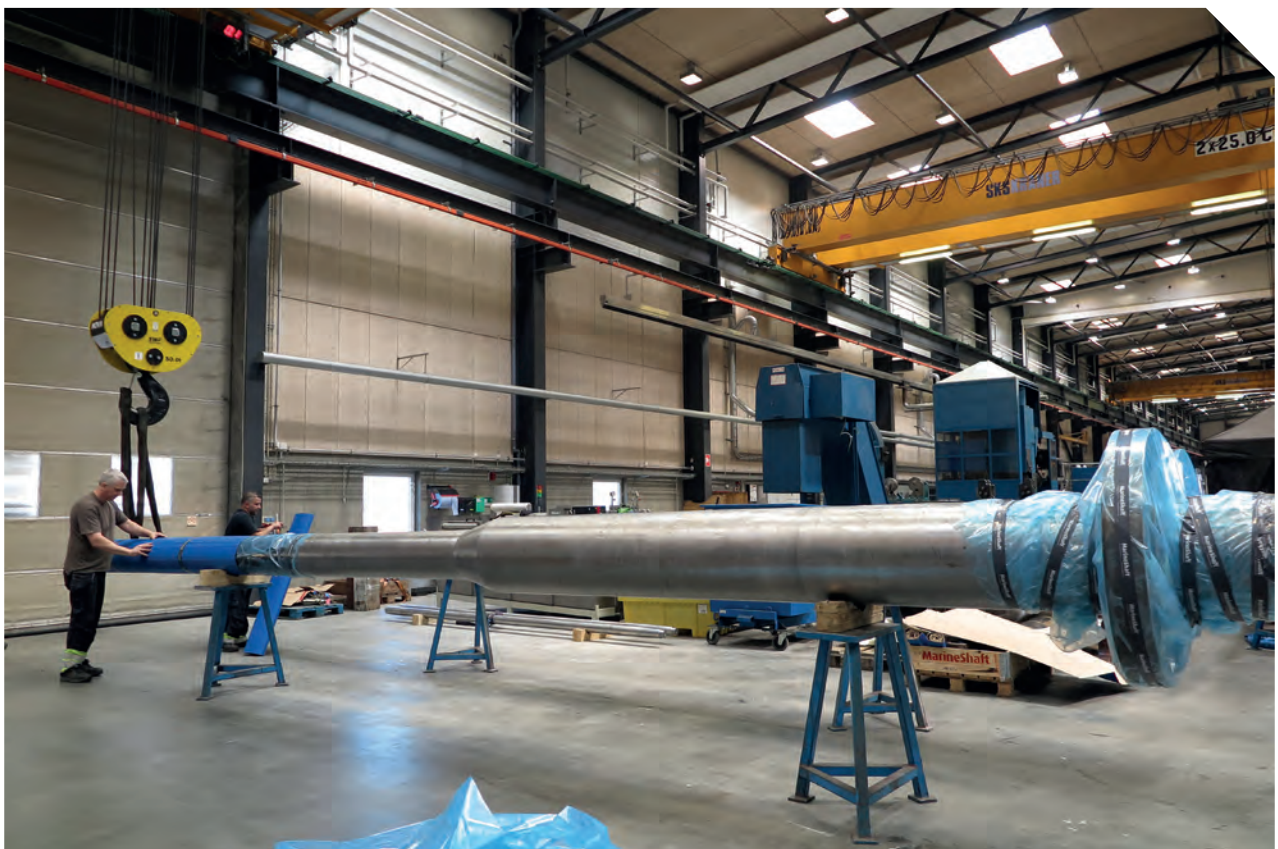
The bent shafts were straightened, corrosion protected, packed with an anti-rust film and wrapped before being loaded onto the truck for safe transport back to the ship
